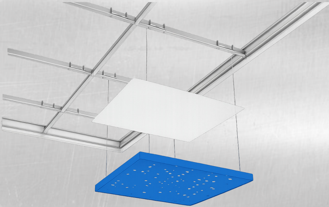
Exploded view of the Perforate panel / PET infill / Grid with saddle clip stack
